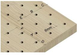
A = 32mm B = 32mm E = 16mm C = 20mm D = 20mm F = 16mm
